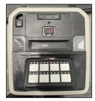
9. Route the small ethernet cable through the hole from step 6 and plug it into the Tundra sPOD switch panel assembly. With the provided socket head hardware, washers, and 3mm Allen wrench, tighten the assembly into the console through the holes from step 5 (arrowed).
