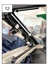
13. Pull the side panel on the driver side end of the dash and remove. Route the ethernet cable from the base of the A Pillar, down to the footwell.
