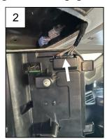
3. Use the flathead screwdriver and pry tool to release the six tabs shown (3a), while applying pulling pressure to the trim panel (arrowed in 3b).
